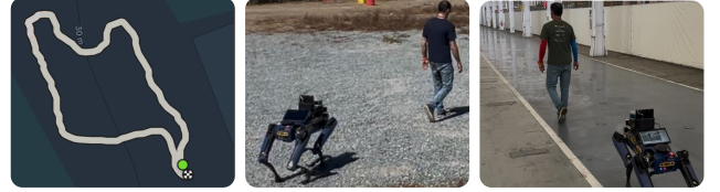
Fig. 10. Left: outdoor route; Middle: robot following on gravel (vision only); Right: indoor following (vision+armbands+Bluetooth).
